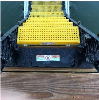
**Step 2** - Remove the two (2) 1/2-13NC button head cap screws and nylon locking nuts from the middle of the folded Step Assembly. Carefully unfold the Step Assembly on a flat surface. Reinsert the screws in the aligned tabs on both sides. Tighten all four (4) 1/2-13 NC button head cap screws and nylon locking nuts.
