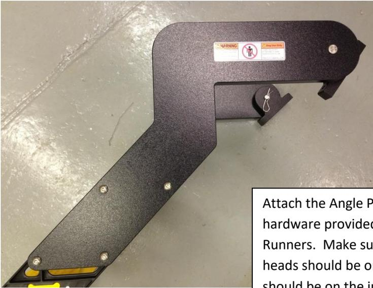
Attach the Angle Pivot Plates to each side of the Step Assembly using the hardware provided in the holes it was shipped in; top four (4) holes in the Runners. Make sure the warning labels are facing outward. The screw heads should be on the outside and the washers and nylon locking nuts should be on the inside of the assembly. Tighten securely. Attach the Pivot Mounts to the Angle Pivot Plates using the Clevis Pivot Pins and Hair Pin Cotter.
