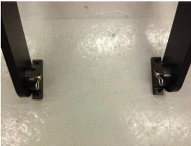
The Pivot Mounts are shown installed on the inside of the Angle Pivot Plates. If preferred, they can be moved to the outside.
