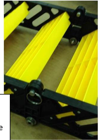
**Step 2** - On a flat surface, remove the two (2) Quick-Release Pins in the folded Step Assemblies, carefully unfold them flat, and re-insert the quick release pins in the holes between the Upper Step Assembly and the Lower Step Assembly. Do not twist the Step Assemblies while unfolding.
